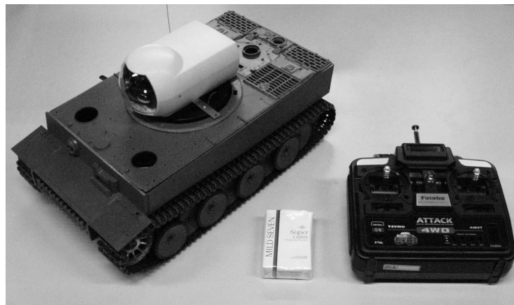
Fig. 1. Picture of the robot : CCD camera on the main body
